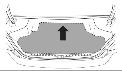
Remove styrofoam floor spacers - Left, center, right side pieces.
