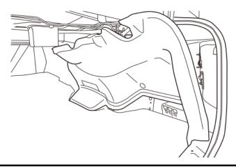
Release the harness clip and disconnect the taillight connector.
